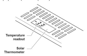
The **temperature readout** ① is located on the **air-inlet grille** ①. It can be programmed and serviced by using the provided remote control.
